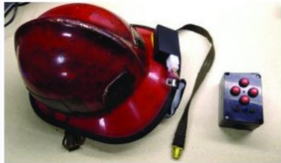
Fig. 5: Helmet with embedded haptic interface in its harness and remote controller.
